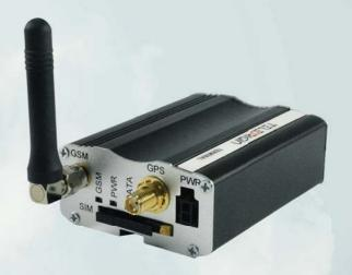
Typical applications of **miniGPSeye** and **RB900-GPS** include fleet management systems, European GPS-assisted road tolling systems, cellular base stations, in-car navigation systems, automotive telematic systems etc.
